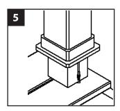
8. Place the bracket against the post with the wire hole lined up to the hole drilled in the post. Secure the bracket down with #6 wood screws or #6 self tapping screws for an aluminum post.
