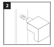
4. Feed the wire from the light through the hole in the post sleeve. Feed the bottom of the post sleeve though the post sleeve skirt. Carefully while holding the wire out of the way at the bottom slide the post sleeve and skirt assembly over the wooden post.
