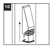
NOTE: If railing has already been installed, lead wires will need to be fished through the post sleeve to reach the desired location for the deck rail light. In some cases the provided lead wire does not fit (due to connector size), the wire connectors can be cut off and wire nuts can be used. Test lights with the power on. If lights wired with this method do not function, switch the connector wires.
